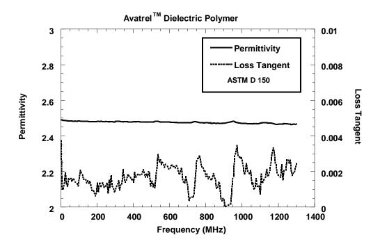
Figure 1: Permittivity and Loss Tangent for Avatrel<sup>™</sup> Dielectric Polymer
