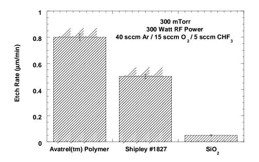
Figure 3: Etch Rate Comparison of Avatrel<sup>TM</sup> Polymer to Soft (photoresist) and Hard (SiO<sub>2</sub>) Mask Etch Rates
