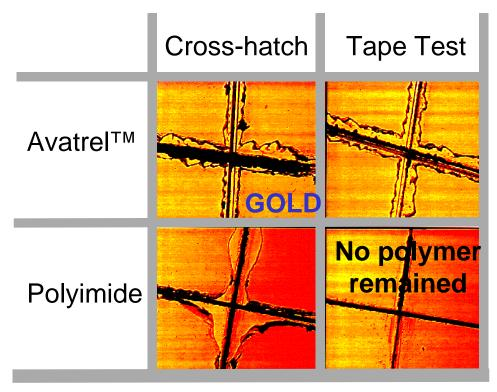
Figure 2: Adhesion of Avatrel<sup>TM</sup> Dielectric Polymer on a sputtered gold surface compared to a typical polyimide
