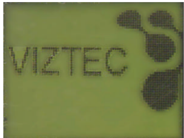
Figure 3. Flexible 96x65 pixel 1.5 inch diagonal monochrome STN display manufactured by Viztec Inc.
