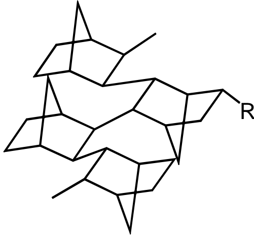
Figure 1. chemical structure of polynorbornene with functional group.
