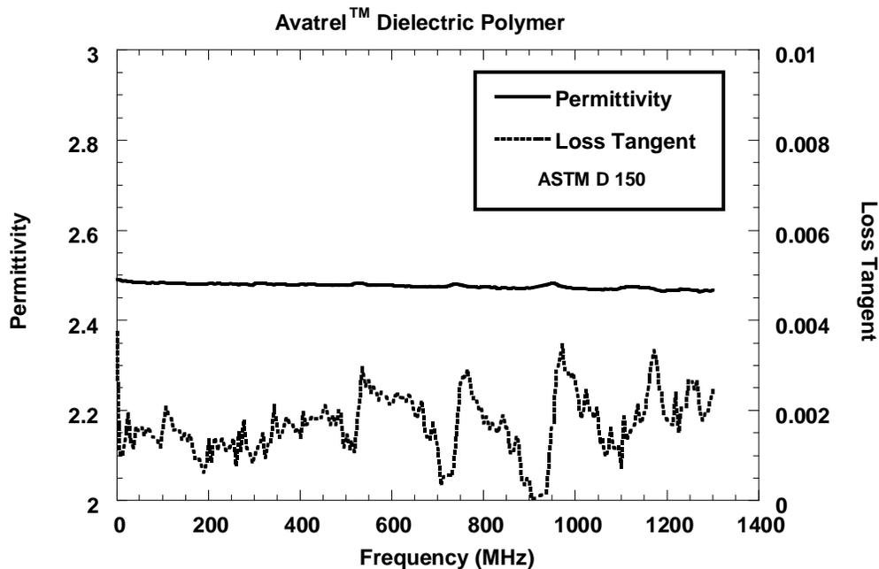
Figure 1: Permittivity and Loss Tangent for Avatrel™ Dielectric Polymer
