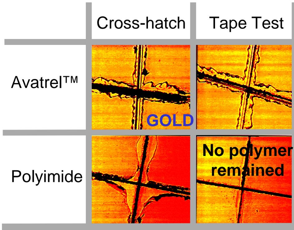
**Figure 2: Adhesion of Avatrel™ Dielectric Polymer on a sputtered gold surface compared to a typical polyimide**
