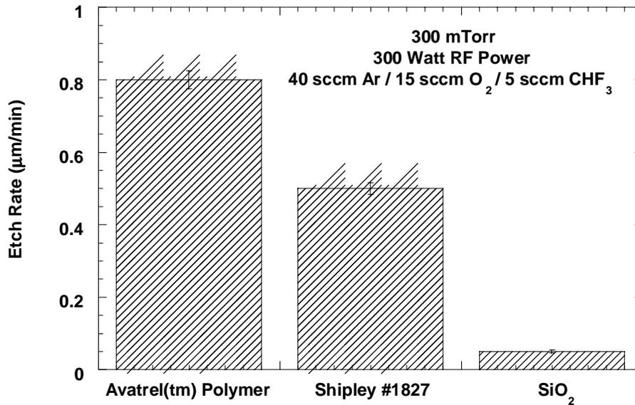
**Figure 3: Etch Rate Comparison of Avatrel™ Polymer to Soft (photoresist) and Hard (SiO<sub>2</sub>) Mask Etch Rates**
